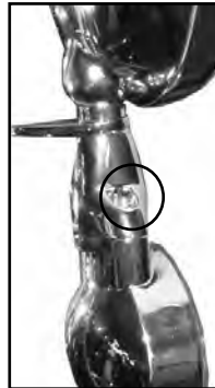
Figure 1. Attach Turn Signal with 10-24 Screws.
